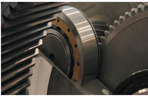
Figure 2: Important lubrication points in wind turbines are in the main gear drive, the yaw system gear, the main and generator bearing, the pitch adjustment unit and the nacelle slewing ring.
